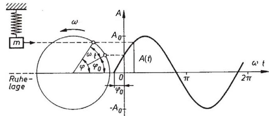
$$A(t) = A_0 \sin(\omega t + \varphi_0) \quad \text{falls } A_{t=0} = 0, \text{ dann } \varphi_0 = 0$$
